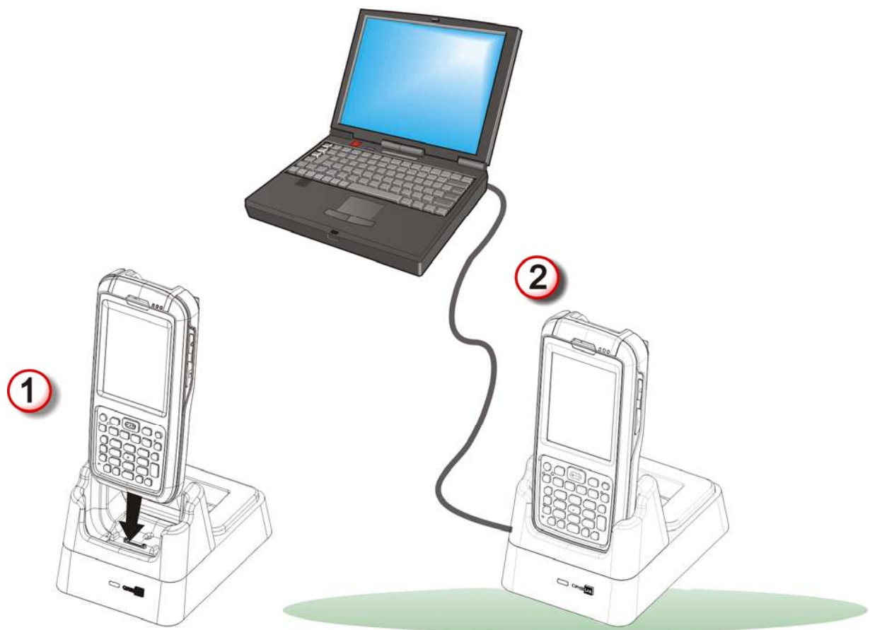
Figure 12: Direct Data Communication Using Cradle
