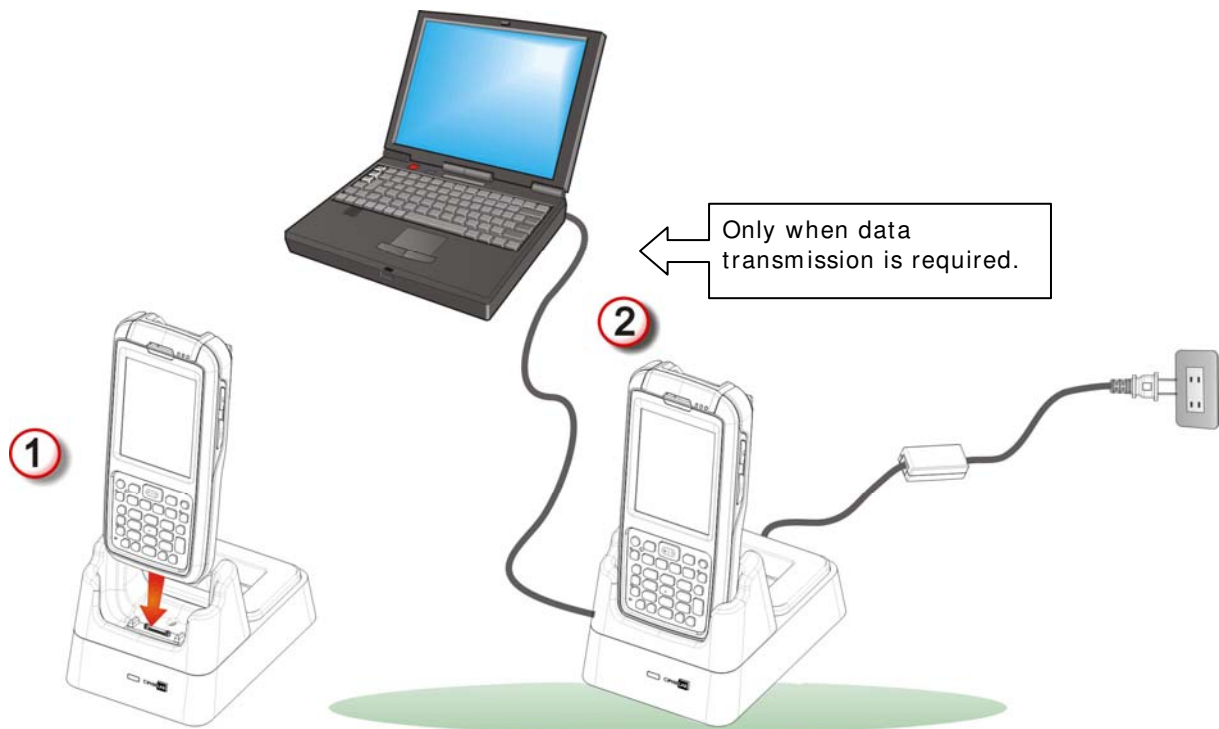
Figure 6: Direct Charging Using Cradle
